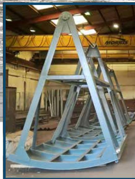
ECS was contracted to produce one 2.38m wide x 1.13m high and eight 2.68m wide x 4.43m high radial gates for installation by their in-house engineers at the weir. The entire design process of each gate was carried out in-house by ECS, with all designs adhering to BS EN 1090-2 certification. The gates were required to geometrically match the existing gates at the weir and mirror their crest level, preserving the water dynamics through the weir.
