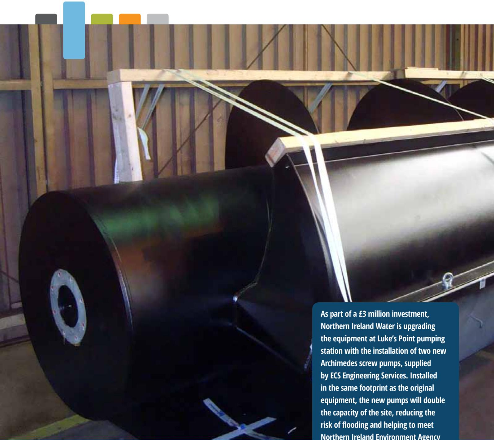
As part of a £3 million investment, Northern Ireland Water is upgrading the equipment at Luke's Point pumping station with the installation of two new Archimedes screw pumps, supplied by ECS Engineering Services. Installed in the same footprint as the original equipment, the new pumps will double the capacity of the site, reducing the risk of flooding and helping to meet Northern Ireland Environment Agency standards for water quality.
