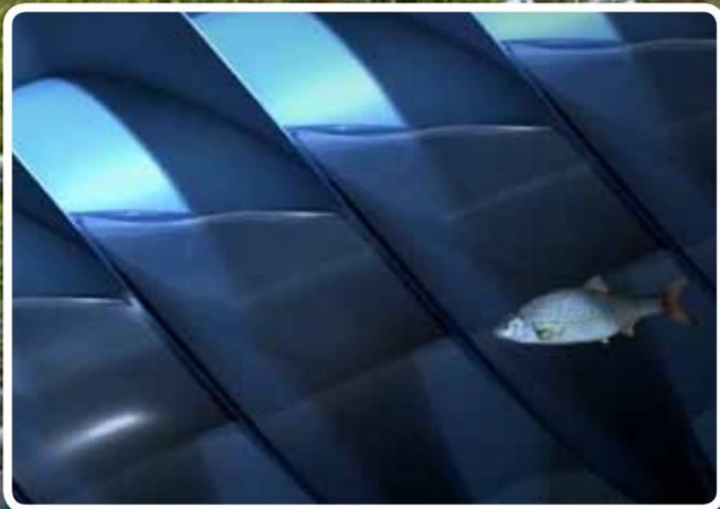
The new screw pump incorporates Landustrie's fish-friendly design that has been proven to allow 98% of fish to pass through unharmed
