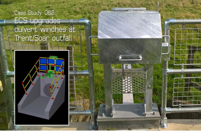
The flaps are made of stainless steel so that they have the durability to survive and provide a long working life in a wet, outdoor location. This makes them heavy, and while most can be opened manually by a single person, the health and safety issues this creates — especially for lone workers — are considerable.
