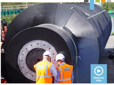
"As part of this contract, we also made new side profiles," says Jake Laughton, who managed the project for ECS. "The replacement pump bodies were almost identical to the original design, but we used finite element analysis techniques to optimise them for withstanding the pumping pressure based on new standards."
