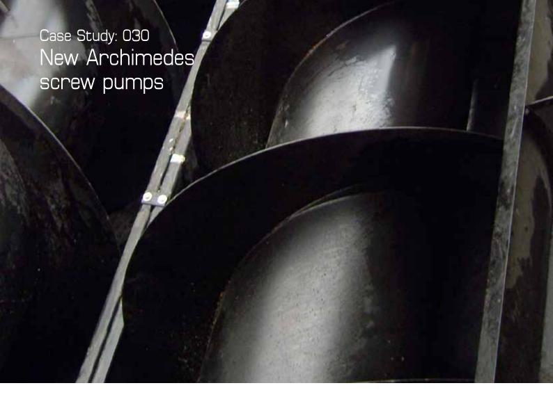
The existing screw pump arrangement at Luke's Point had reached the end of its design life and was no longer efficient. The screws themselves were heavily worn and the drive system was in need of improvement in terms of efficiency and reliability. As a result, a contract was issued for the replacement of this equipment and it was awarded, in part, to ECS and its partner Landustrie, a leading manufacturer of Archimedes screw pumps.
